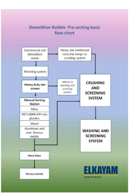
The **ELKAYAM** pre-sorting installation is a complete pre-sorting installation which is designed to be semi-portable and can be employed stand alone or integrated into a crushing washing and screening system, dependent on the demands of the specific job and area.
